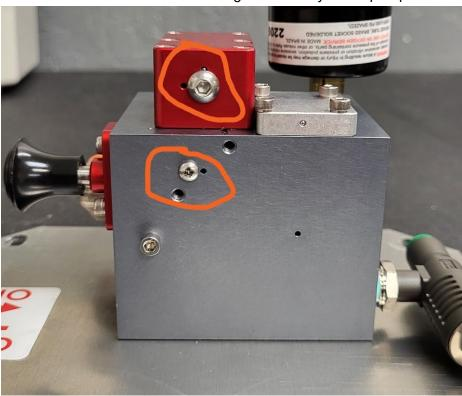
6. Install the silver solenoid into the top hole then use a hex key to tighten
