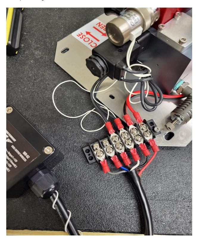
12. Remove the white plastic cover and install a grommet to run your power and ground through then reinstall the control box back into the enclosure.
