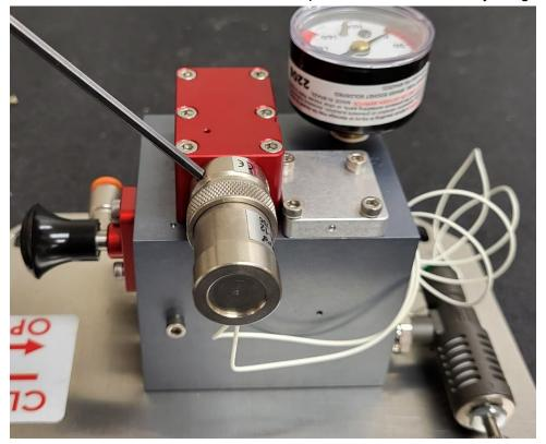
7. Loosen the knurled nut to adjust then retighten
