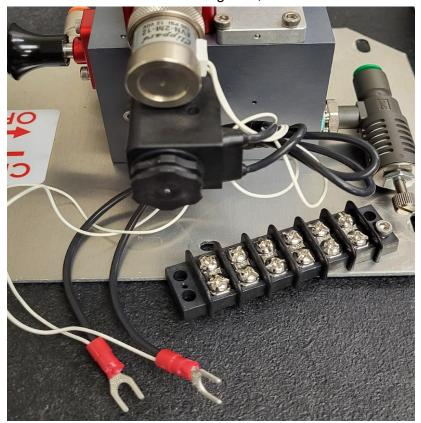
11. Connect the two solenoid wires to the white and brown wire from the receiver, the blue and gray will only be used if you are wiring two boxes together. Red and black are your power and ground wires.
